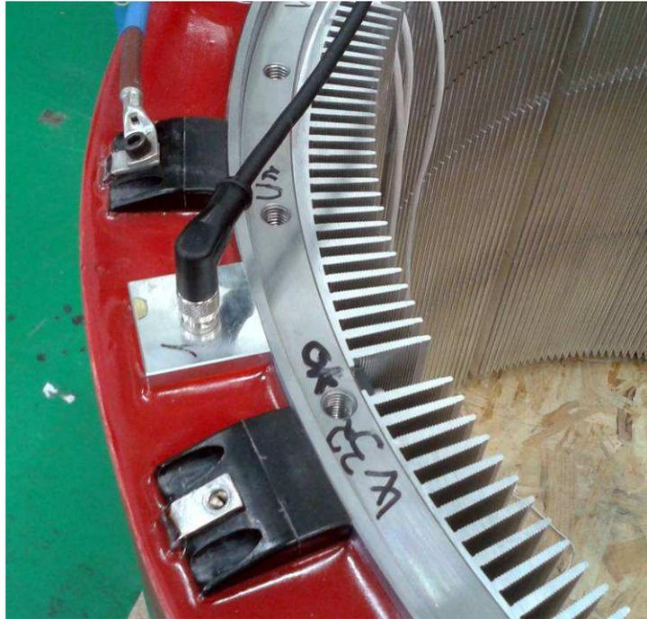
**Figura 7: outside rotor, IP 65 forced air cooled 80,000 Nm motor for DD elevators**
