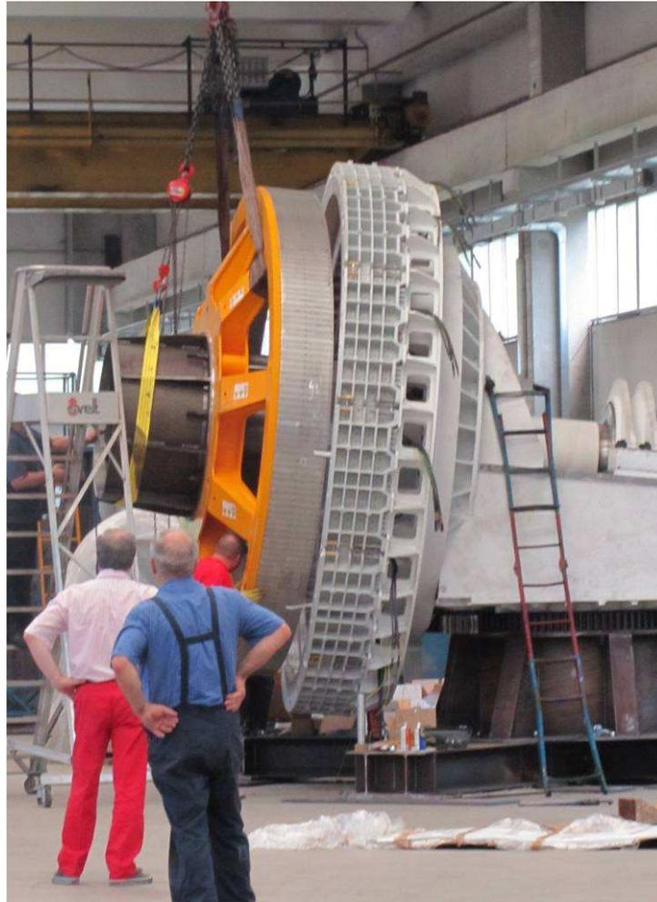
Figura 6: Modular frameless double cylindrical air gap generator, 1 MW, stack = 340 mm
