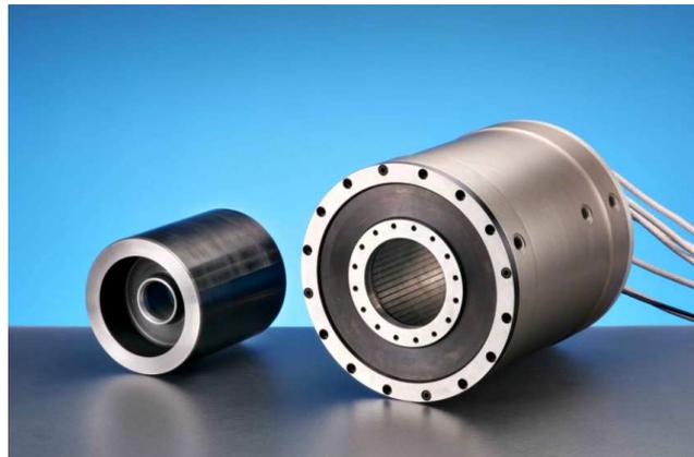
field orientation and for position/speed control. The rotor is permanent magnet type and has no primary losses, so that no rotor cooling is needed in principle. However, the inverter chopper frequency must be set high enough to ensure that the ripple current, pk-pk is less than 20% of the nominal rms current to avoid the insurgency of unacceptable, and dangerous, stray rotor loss.
