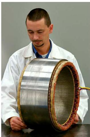
**A three phase stator**, wound and vacuum encapsulated in super high thermal conductivity compound (for low surface temperature operation) or impregnated (3 dips, preferred solution for high thermal cycling), which is either built into a metallic frame carrying the cooling chambers and coupling O-Rings on the outside and a set of tapped holes on one side (SQUID type), or into a thin steel microframe, cylindrical.
