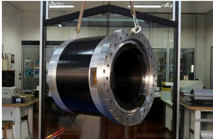
The magnets are generally high temperature, high energy FeNdB sintered magnets, Phase Motion Control manufactured with a special patented technology. They are designed for the maximum class
