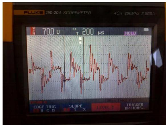
To limit such voltage transients, Phase supplies with each motor with such characteristics a tuned anti resonance filter (snubber) which must be assembled within 5 m of the motors, between the motor star terminal (white wire) and machine ground. Failure to connect the snubber may result in motor failure by insulator puncturing. Phase can supply different type of snubber depending on motor size.
