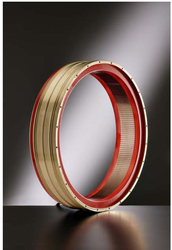
Customized frames with integral cooling or even partial machine subassemblies with bearings and encoders are manufactured on request based on the standard frameless magnetic designs available. The torque range spans from 10 to 40,000 Nm with maximum diameter 1150mm; above that size, segmented semi custom units are available, currently up to 18 m diameter.
