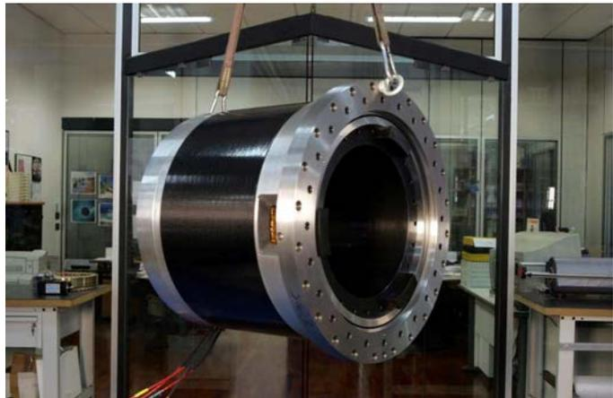
The magnets are generally high temperature, high energy FeNdB sintered magnets, Phase Motion Control manufactured with a special patented technology. They are designed for the maximum class temperature and are virtually impossible to demagnetise except in case of drive failure or improper operation. If continuous exposure to oil is forecast, special oil resistant magnets can be specified.
