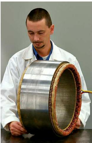
**A three phase stator**, wound and impregnated (3 dips, preferred solution for high thermal cycling), or vacuum encapsulated in super high thermal conductivity compound (for low surface temperature operation), which is either built into a thin steel microframe, cylindrical, or into a metallic frame carrying the cooling chambers and coupling O-Rings on the outside and a set of tapped holes on one side (Squid type).
